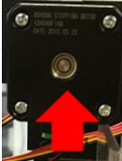
9. Remove the coupler and X motor from printer.
