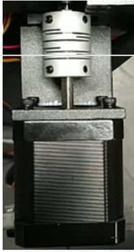
13. Hold the X motor in place and pre-tighten the four screws which secure the motor on frame.
