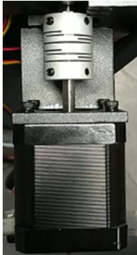
15. Hold the motor still on that position and tighten all screws on the frame.
