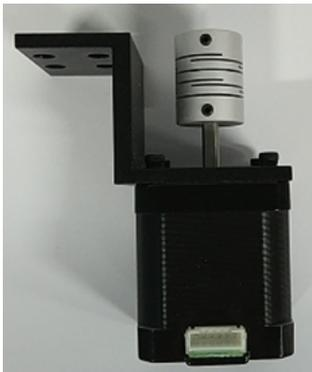
Note: Rotate the coupler slightly until one of its grub screws are over the flat surface on X Motor Shaft.
